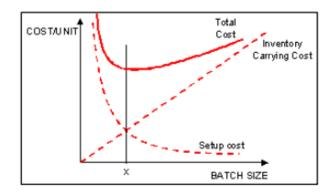
In the above diagram, it is shown that the x-axis is batch size and the cost of a unit is on the y-axis. It is shown that with the increase in batch size holding costs also tend to increase whereas setup costs tend to decrease. The point where both the cost line intersects each other signifies the lowest cost combination. The objective is to determine the batch size that developed on both sets of formulas.
